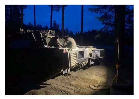
Figure 3. Mechanics from Assault Company, 1<sup>st</sup> Battalion, 8<sup>th</sup> Cavalry Regiment's field maintenance team conduct battle damage assessment repair on an M1A2 SEPv3 Abrams tank during Operation Lock, May 2023. (Army photo by 1LT Raven Parker, battalion unit public affairs representative)
